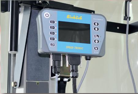
Power is supplied via the tractor's on-board electronics. Via the **7-pin signal socket**, sensor values of the tractor can be taken over (e.g. speed)
