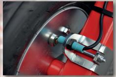
A wheel sensor measures the speed at one wheel of the attachment.
