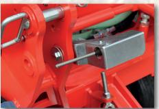
A 3-point-linkage sensor automatically switches off the sowing roller when the implement is lifted.
