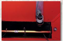
The level sensor signals when the tank is getting empty. The sensor works inductively and is therefore independent from vibrations.
