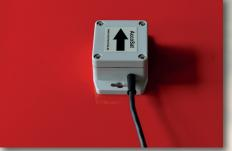
The GPS sensor on the tank is an option to determine the speed precisely.
