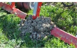
The **triangular front levelling plate** of the PRO-series
