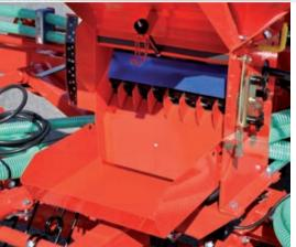
The **calibration pan** and cover are standard on the machines.
