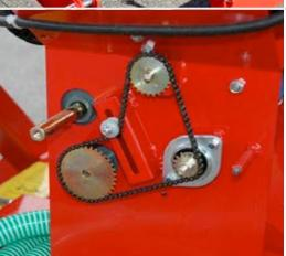
A **chain with tensioner** connects the infinitely variable oil bath gearbox (or the electric seeding roller motor) with the seeding roller and the stirring shaft.
