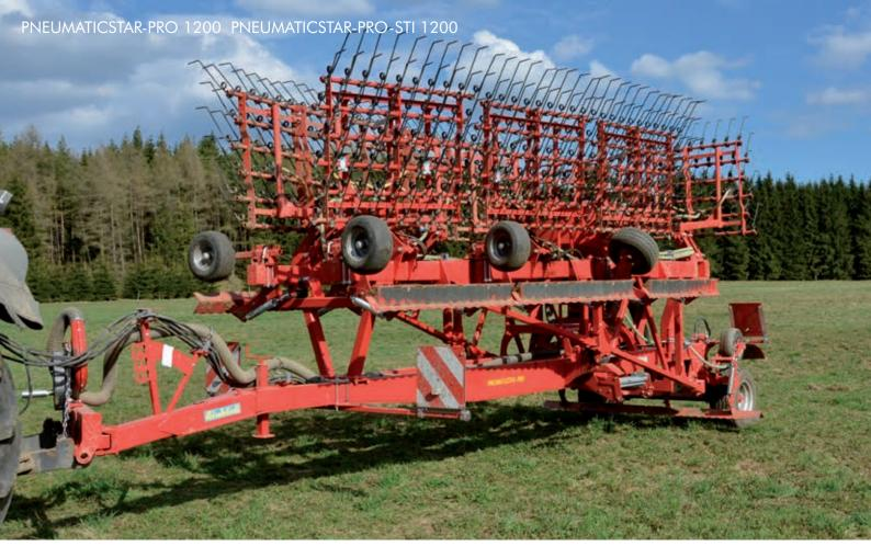
The sophisticated **retraction mechanism** together with putting the tines into the lowest angle position makes it possible to reduce the transport width to only 3 m
