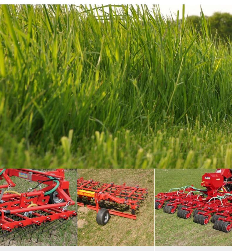
The hydraulic tine adjustment makes adjustment to the GRASS-MANAGER, PNEUMATICSTAR and PNEUMATICSTAR-STI in changing soil conditions easier. Also, folding to the transport position is more convenient as you can easily put the tines into a flat position. The hydraulic tine adjustment can be retro-fitted.
