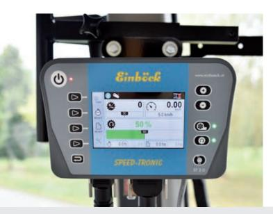
The PNEUMATICSTAR and the PNEUMATICSTAR-PRO can be equipped with the SPEED-TRONIC control unit. Then they are called PNEUMATICSTAR-STI and PNEUMATICSTAR-PRO-STI.
