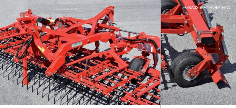
For the PRO-series there is a **front mounting frame** available. Whith this frame an existing rear mounted machine can easily be converted into a front mounted machine.
