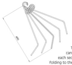
The aggresiveness of the spring tines can be adjusted via a **central lever** per each section in 5 different positions. When folding to the transport position the tines should be adjusted to the flattest position.
