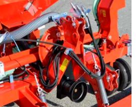
With the **mechanical fan** you can distribute heavier seeds up to 6 m working width due to the higher airstream. You can work with increased working speed. Recommended for communities and contractors.
