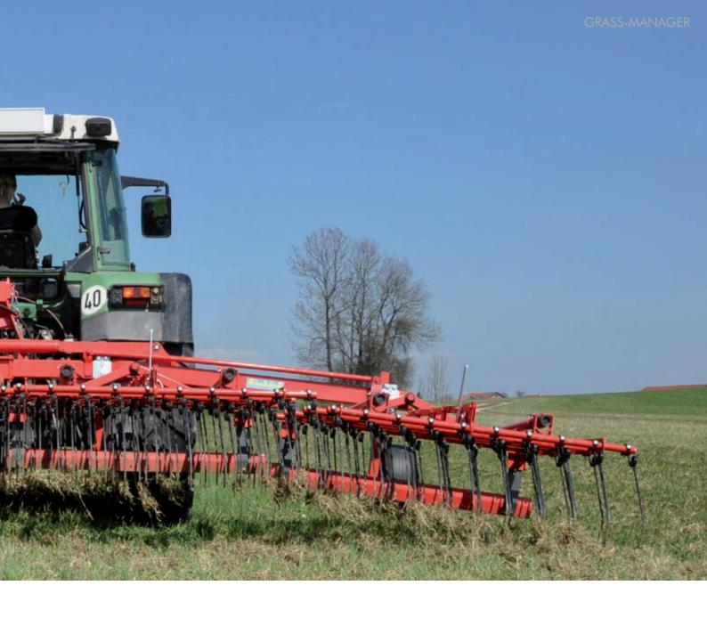
By taking away or demounting the stop bar on the wing (only on machines without shear folding) the machine **follows the contours of the land surface perfectly.**
