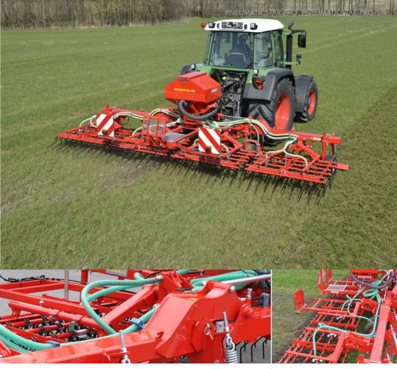
The joints consist of a hardened bolt with 35 mm Ø and brass bushingswhich can be greased.
