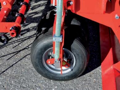
Ground drive via the support wheel (PNEUMATICSTAR). The flexible shaft, which runs a infinitely variable oil bath gearbox, is protected by a hose. The information about working speed is provided from the support wheel. There is no additional ground wheel necessary.
